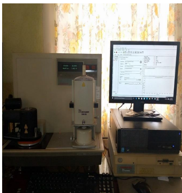
Plate 6: TA Instruments Modulated Differential Scanning Calorimeter MDSC 2920/DTA 1600
