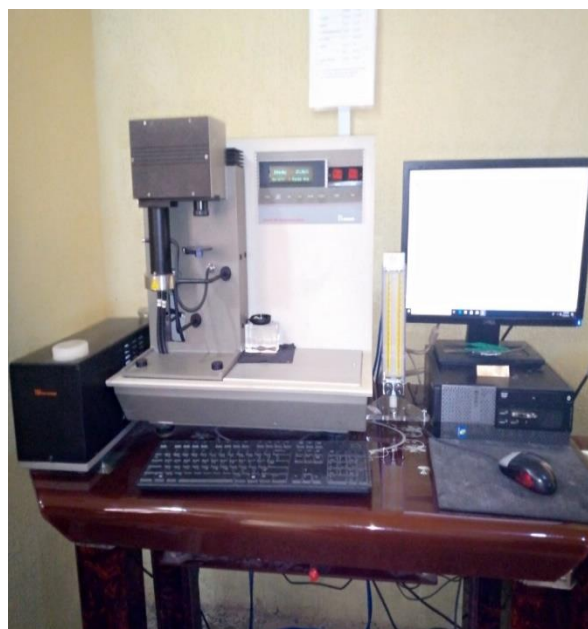
Plate 7: TA Instruments Thermogravimetric Analyzer TGA 2950
