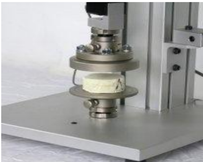
Plate 2: Compression test system outlay (TestResources, 2021)
