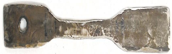
Plate 1; specimen sample used for the Tensile test (Material: Stainless steel 316L)
