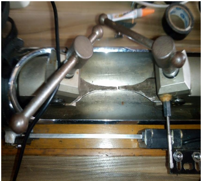
Plate 8: The Tensile test being conducted at an Engineering Laboratory at PGI Applied Resources (Nigeria) Limited
